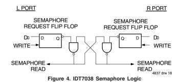
over to the other side as soon as a one is written into the first side's request latch. The second side's flag will now stay LOW until its semaphore request latch is written to a one. From this it is easy to understand that, if a semaphore is requested and the processor which requested it no longer needs the resource, the entire system can hang up until a one is written into that semaphore request latch.
